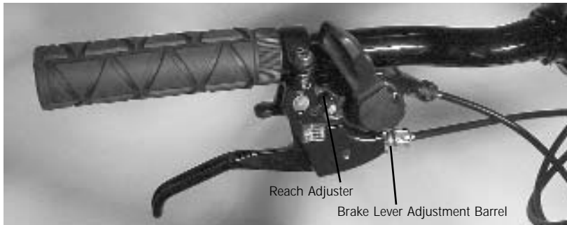
FIGURE 8 - Lever. On some brake levers, the reach adjuster is on the rear side of the lever and is adjusted with a 2mm allen key or flathead screwdriver.
