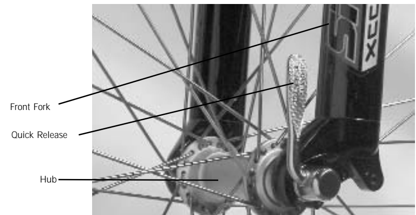
FIGURE 3 - Front hub quick release in closed position.
